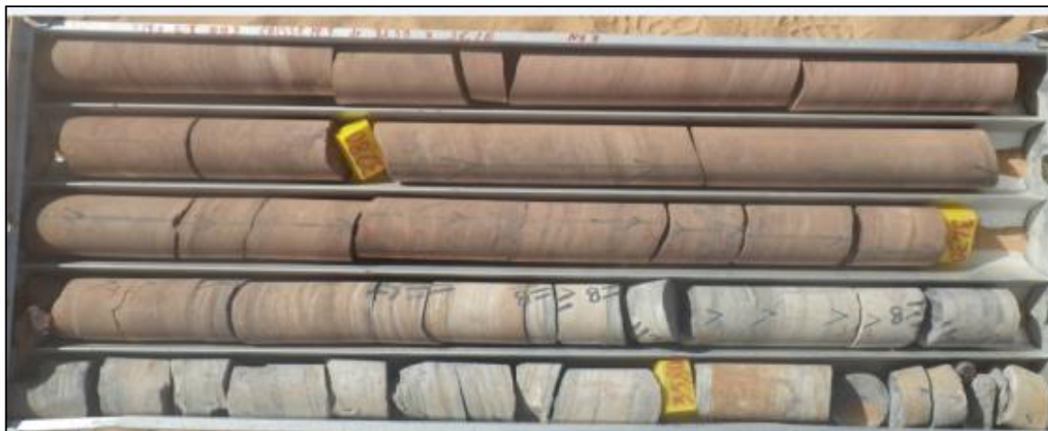
Figure 7-3: Oxidation and weakening of the Tchinezogue unit due to exposure above the water table. Below the water table (approximately 35 m depth) the rock is generally unweathered.
