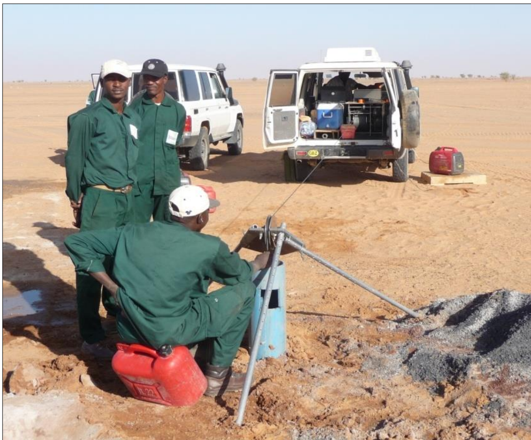
Figure 11-1: Down-hole gamma logging at Madaouela
