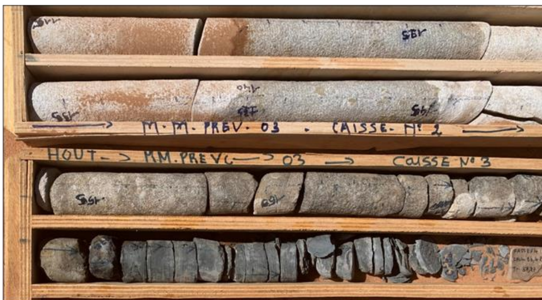
Figure 12-5: Guezouman contact with Talak shale. Base of Guezouman is relatively coarse grained, approaching conglomerate, and accompanied by intensification of mineralisation (strong scintillometer response).
