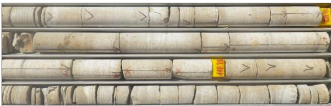
Figure 7-4: Guezouman sandstone showing a zone of relatively closely spaced bedding planes
