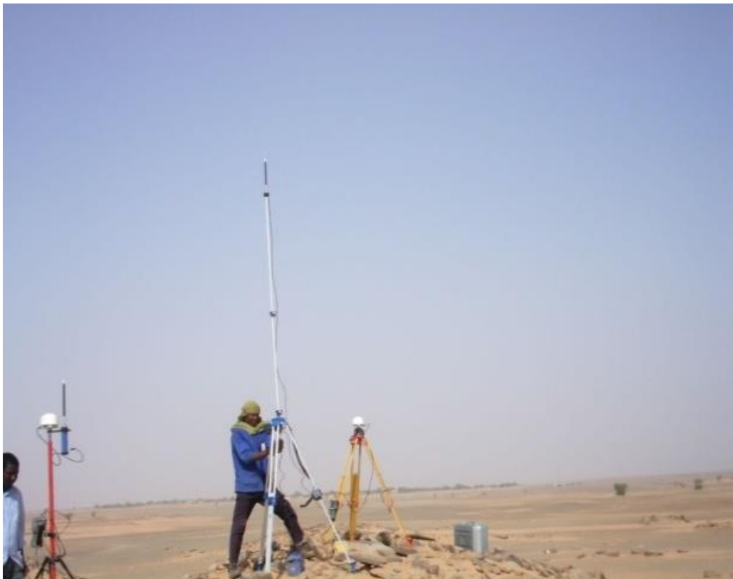
Figure 10-11: Digital GPS surveying in the field; reference and rover
