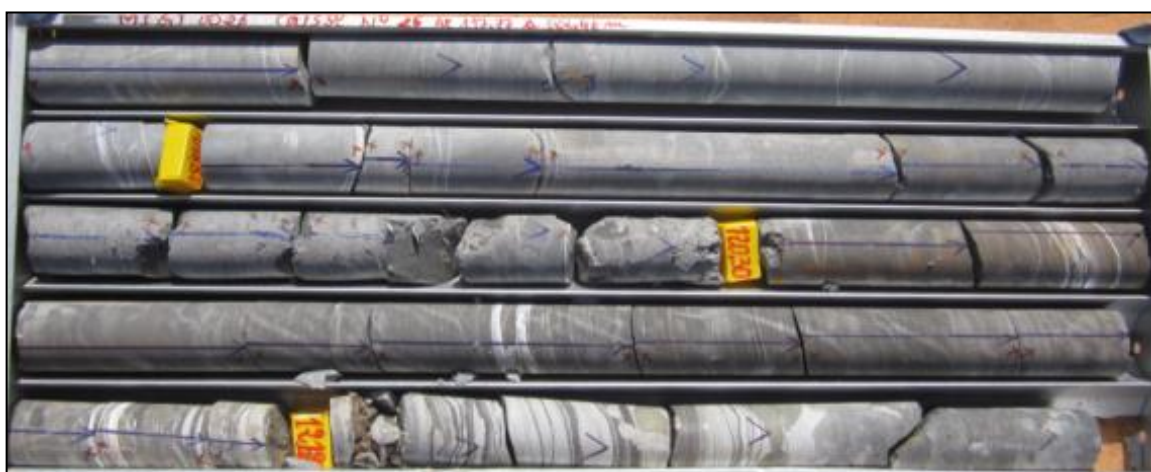
Figure 7-5: Example of the Talak argillite at Miriam (this will form the floor of the pit)
