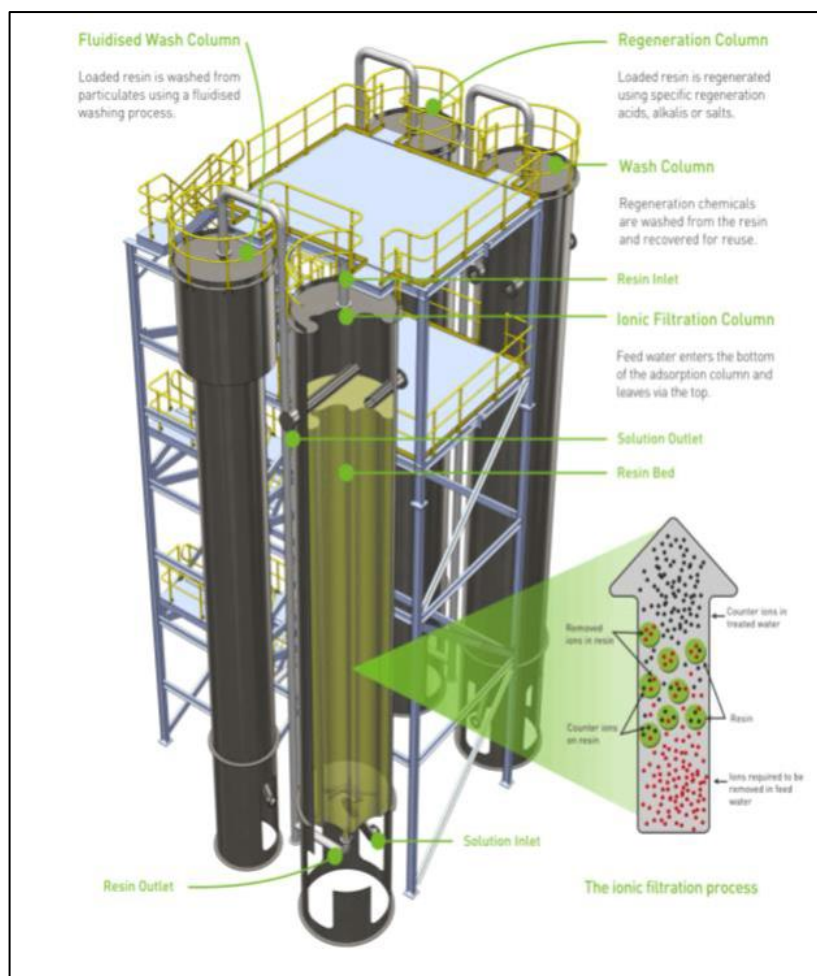
Figure 17-3: Simplified schematic diagram of a typical CIX process
