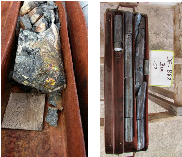
Figure 3: Chalcopyrite and quartz in fault zone at end of Hole DF-565 (left) and Hole DF-882 (right).
