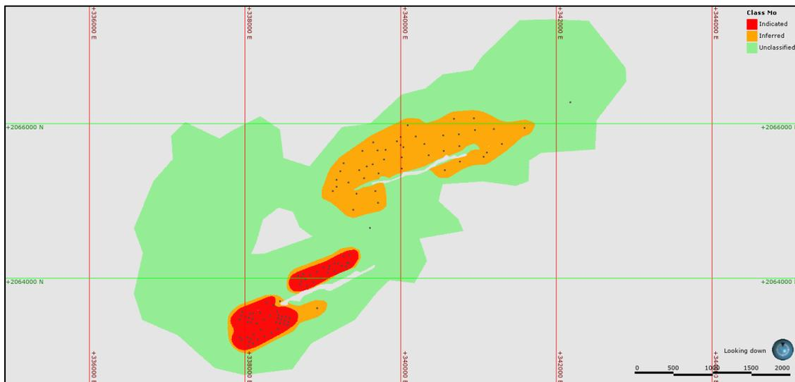
Figure 3: M&M deposit coloured by classification for Molybdenum
