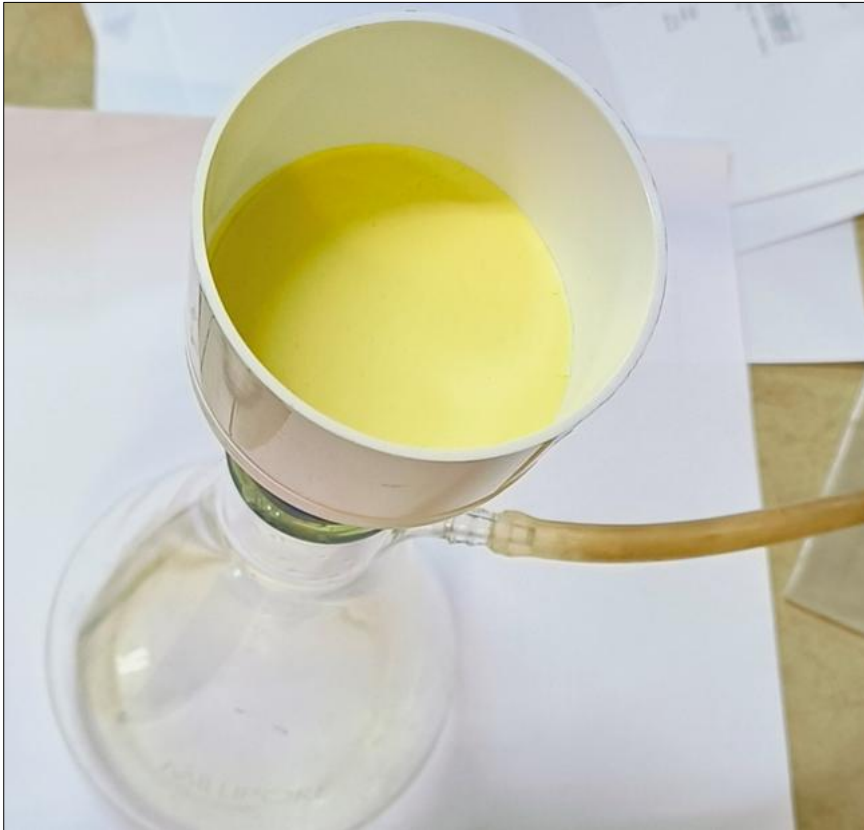
Figure 13-53: Uranium precipitation test
