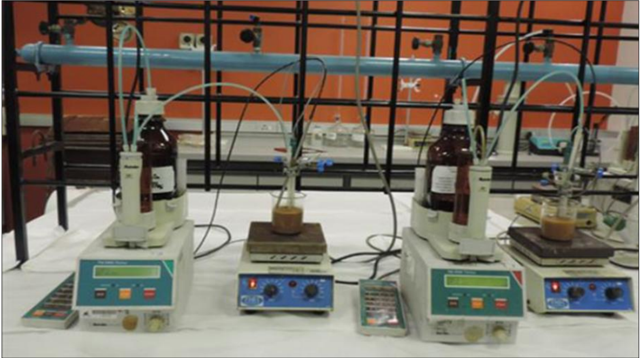
Figure 13-17: Setup, iso-pH test
