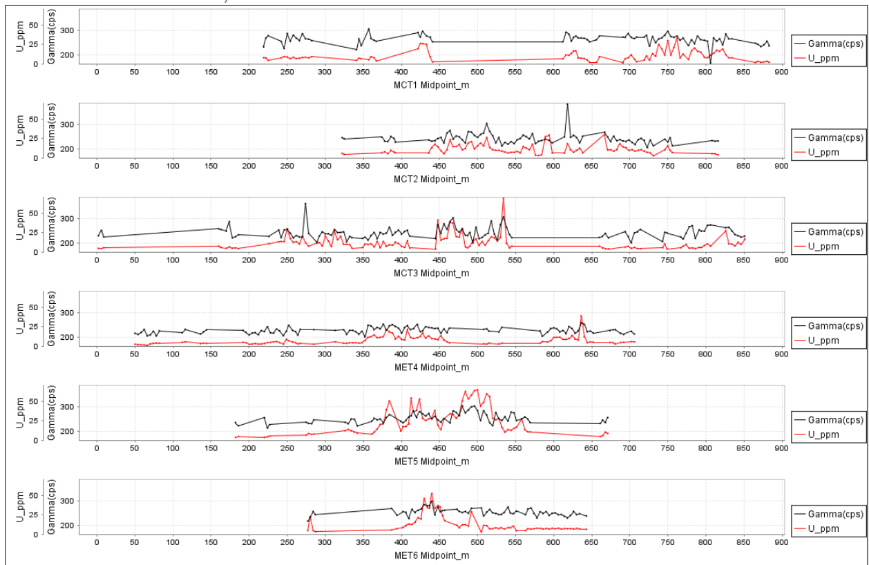
Figure 9-12: Uranium assay and sample total Gamma readings for 2014 trenches (0 m represents the southern end of the trench)
