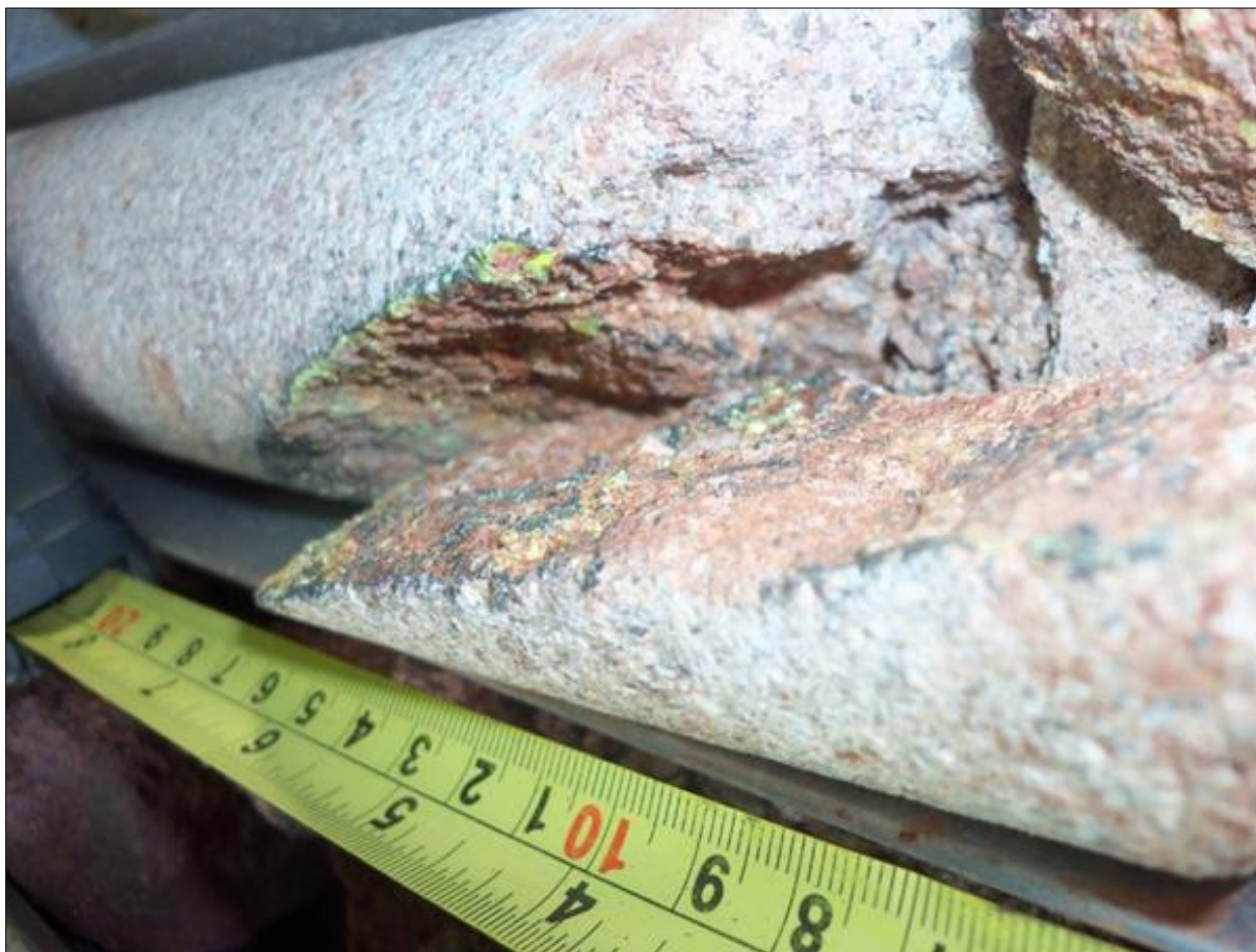
Figure 13-3: Mineralisation in a fracture with the presence of Mn oxide (Source: Denison and RPA, 2012)
