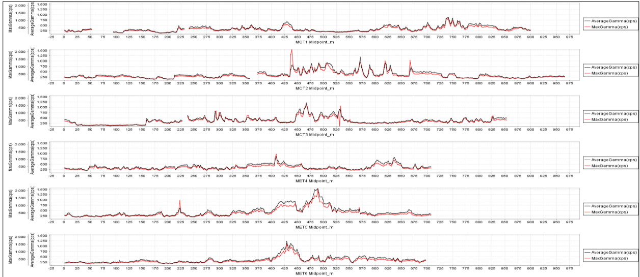
Figure 9-9: Average and maximum total Gamma readings for 2014 trenches (0 m represents the southern end of the trench)
